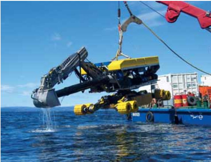
■ The Spider Trenching ROV being retrieved back to the mother vessel
